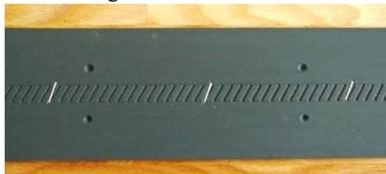
The proofing strip can easily be adapted by means of straight tin snips and a Stanley knife. Crosswise cuts (the red dotted lines) can be made by tin snips while lengthwise cuts (the green dotted line) are best made with a Stanley knife:
