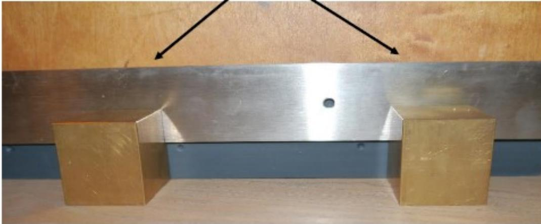
The protection strip is placed in the indentations of the two blocks and thereby elevated from the floor and simultaneously pressed against the proofing strip.
